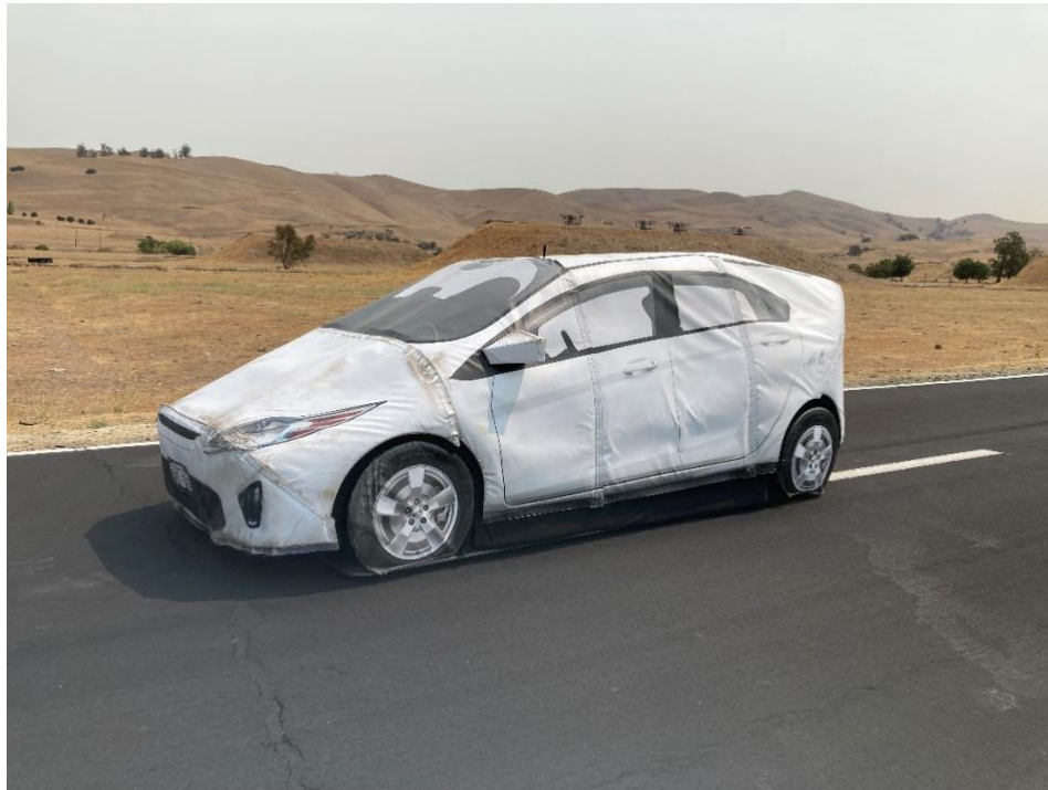
Figure 7: DRI Low Profile Robotic Vehicle. Image Source: AAA
