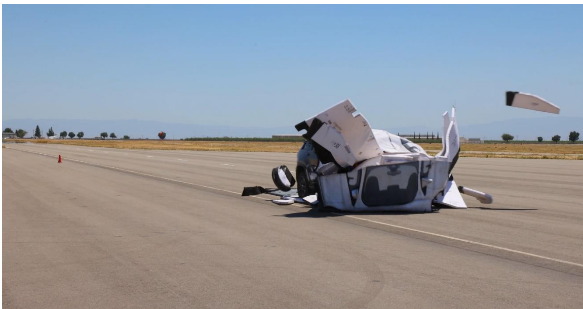
Figure 25: Early Model Jeep Grand Cherokee impact at 35 mph. Image Source: AAA Inc.
