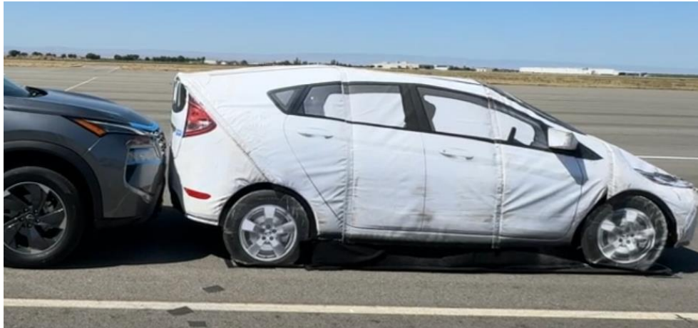
Figure 10: Longitudinal distance zeroing process. Subject vehicle is moved forward until contact is made with the Soft Car 360°. This creates zero-point for distance and TTC calculations. Image Source: AAA Inc.
