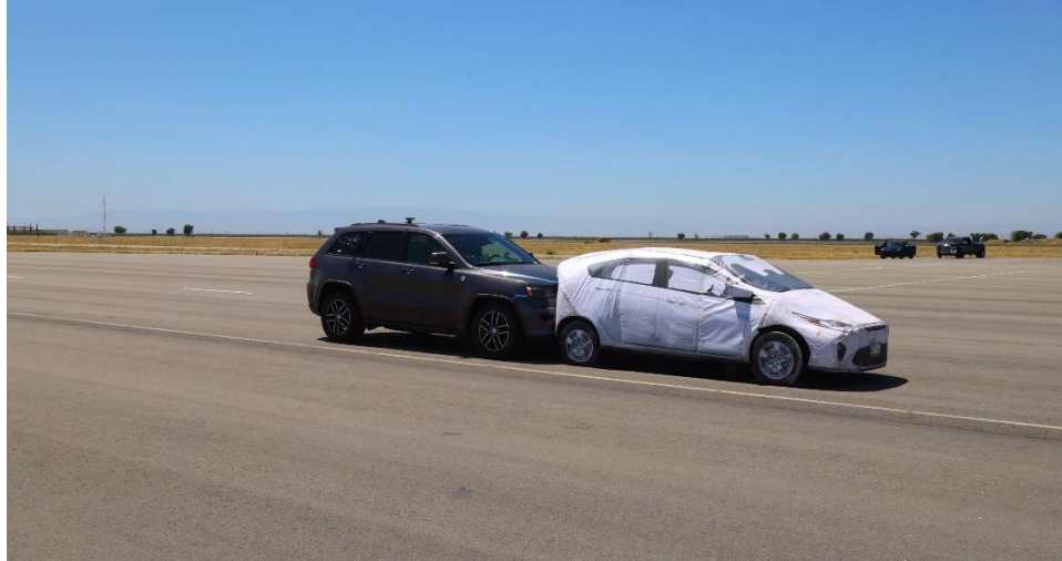
Figure 12: Closed-course test facility with lane markers and Soft Car 360 ® positioned in lane. Image Source: AAA Inc.
