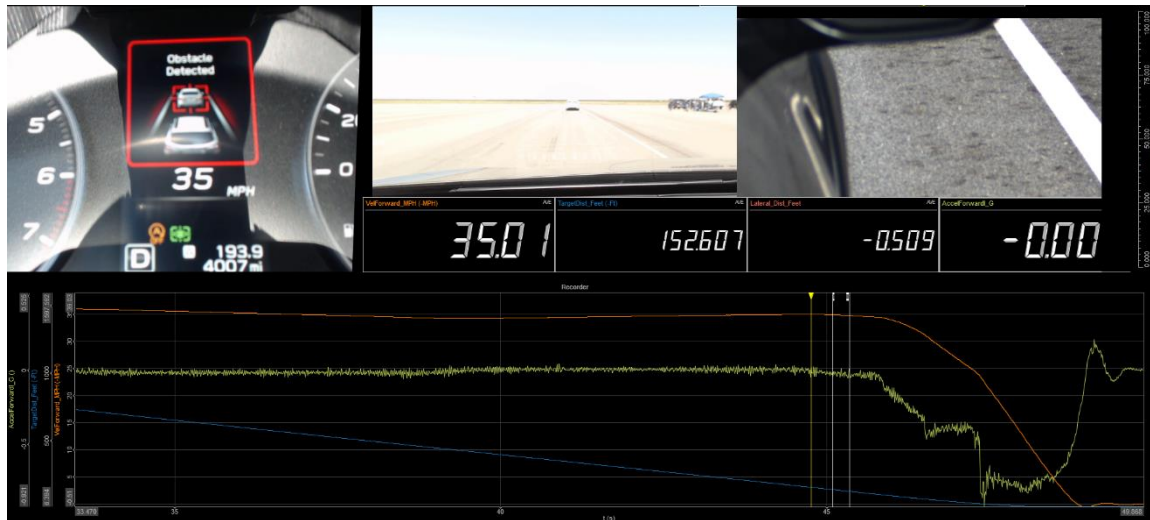
Figure 14: Data Analysis Software with Video and Data Overlay w/ FCW Alert. Image Source: AAA Inc.
