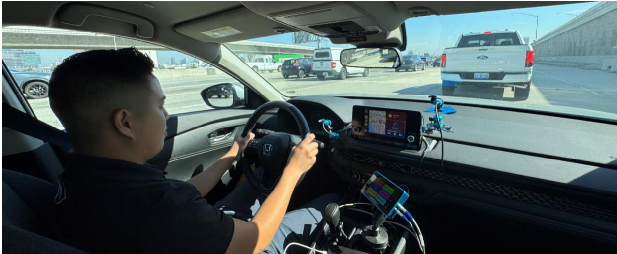
Figure 1: Photo of test vehicle interior during testing, showing touch screen and cameras. Image source: AAA.
